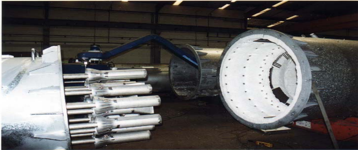
Figure 4 – Ceramic lining inside the flare stack (insulation)
