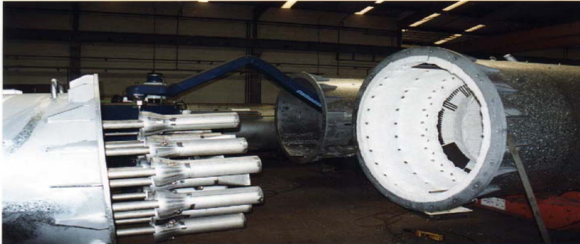
Figure 4 – Ceramic lining inside the flare stack (insulation)
